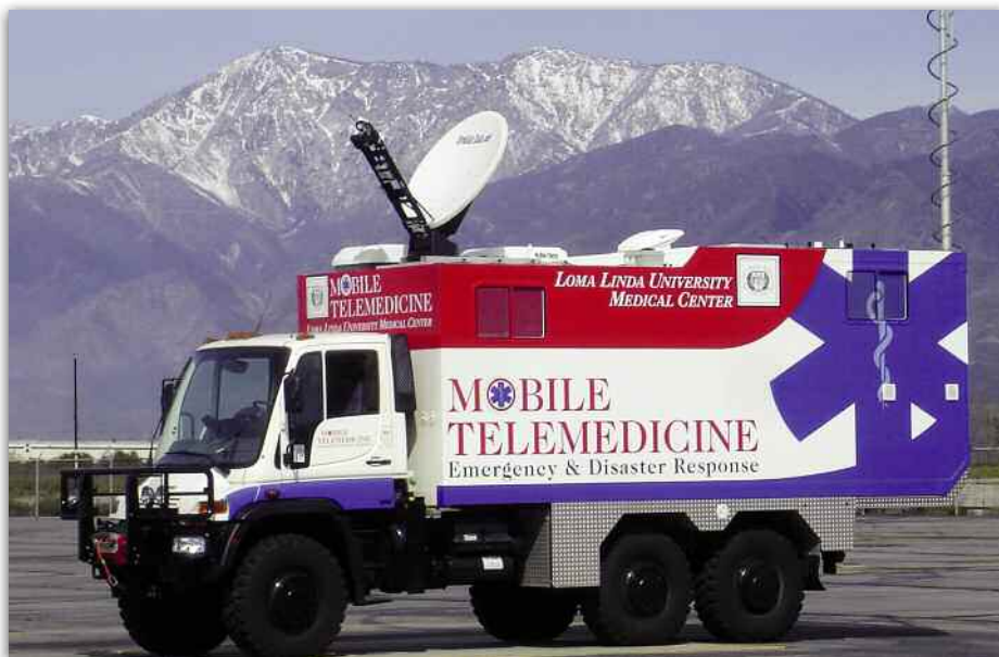
The mobile telemedicine vehicle is designed to reach off-road and remote access areas to extend the expertise of Loma Linda University Medical Center's physicians.
