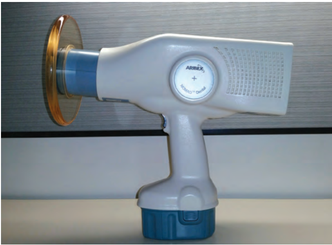
Figure 16. The Aribex Nomad portable hand-held x-ray unit is recommended for use in remote areas where installation of standard intraoral, panoramic, or advanced imaging systems is not possible.
