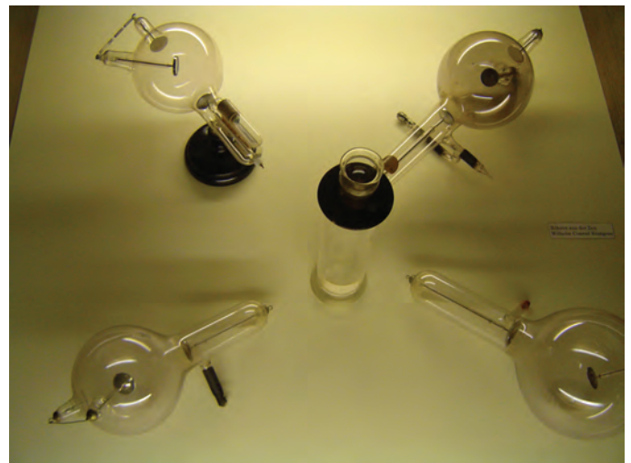
Fig. 1c. Examples of Hittorf-Crookes tubes. These hybrid tubes varied in size, shape and electrode placement. They became the preferred cathode ray tubes for scientists. When applying a voltage potential of up to 49keV, a stream of cathode rays was produced. Much research was dedicated to the properties of cathode rays produced in these tubes by many of the prominent scientists in the latter nineteenth century. This research is what led to the discovery of X rays.
