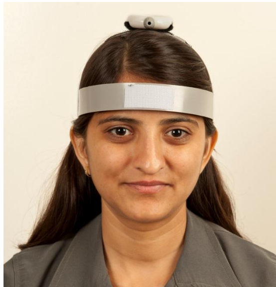
FIGURE 9. Head-mounted laser pointer for joint position error testing.
