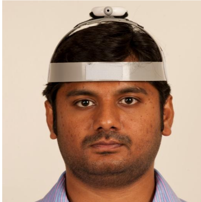
FIGURE 14. Head-mounted laser pointer for joint position error testing.
