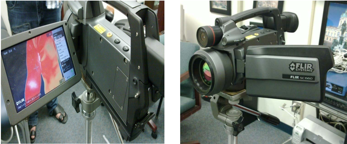
Figure 11. The IR thermal camera used for this investigation (FLIR 660)
