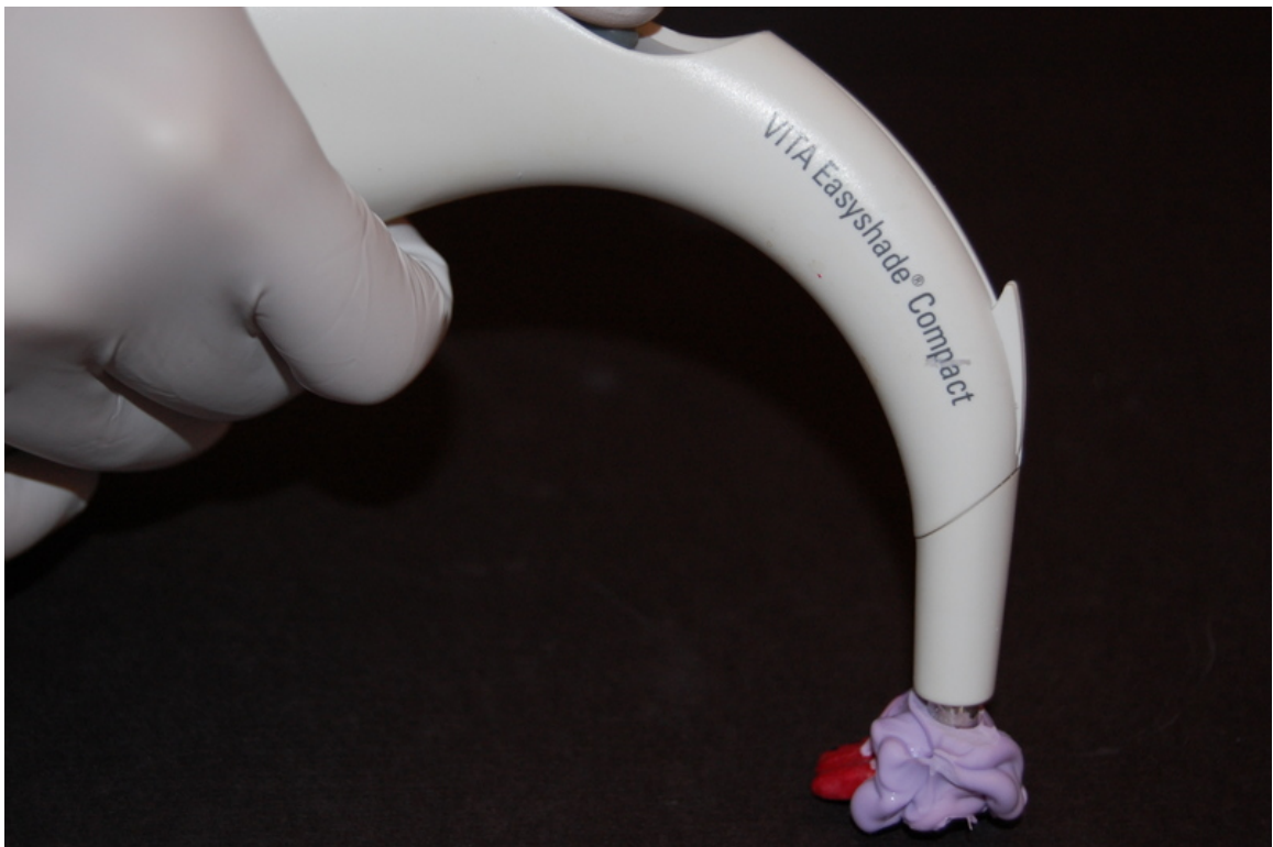
Figure 3: Tip of the spectrophotometer guided by the custom jig to the test area of the tooth specimen
