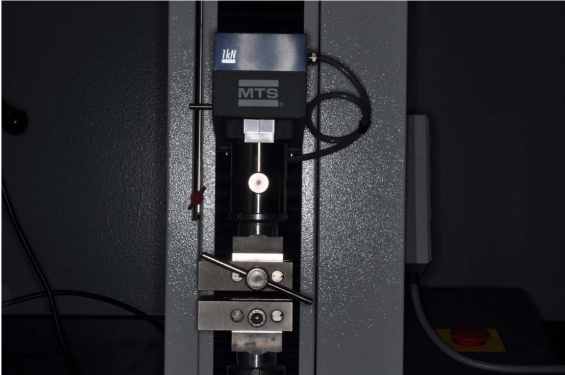
Figure 6. MTS machine was used to complete tensile testing of our bone specimens.
