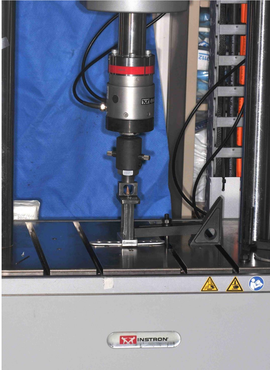
Figure 7. Testing apparatus attached to Instron E10000 machine
