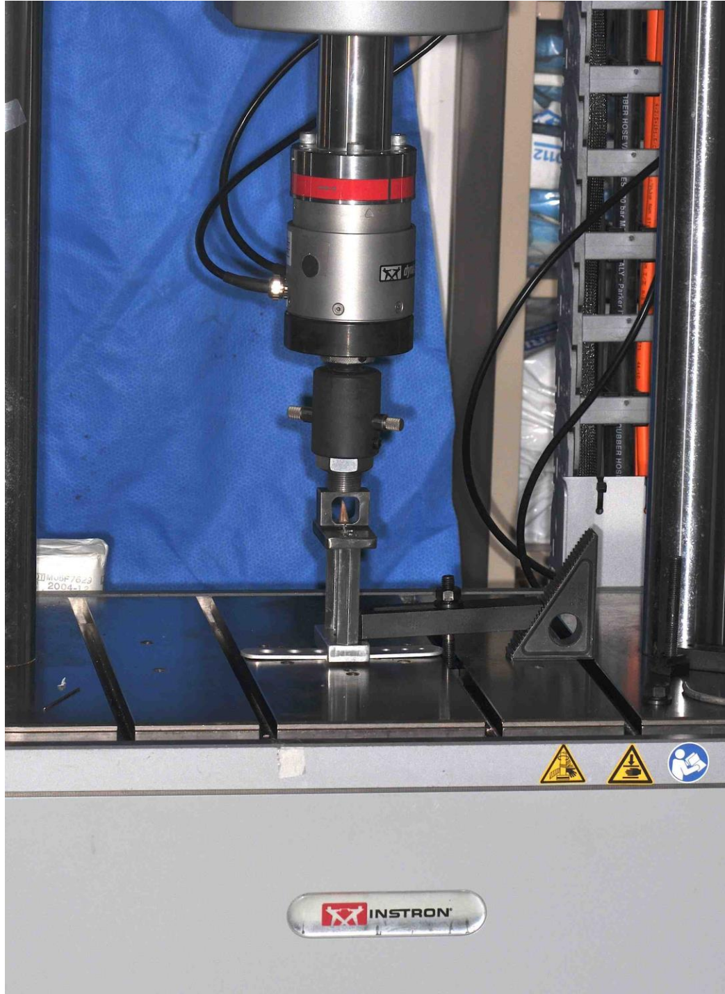
Figure 7. Testing apparatus attached to Instron E10000 machine
