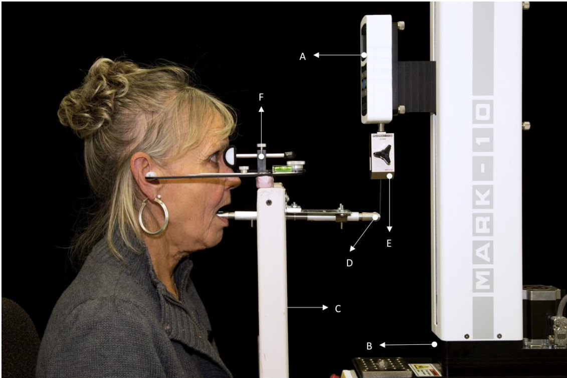
Figure 2. Illustrating testing apparatus. A. DAFG, B. motorized test stand Mark-10 extended length ESM301L, C. wood stand, D. FTD, E. grip attachment, and F. Panadent earbow.
