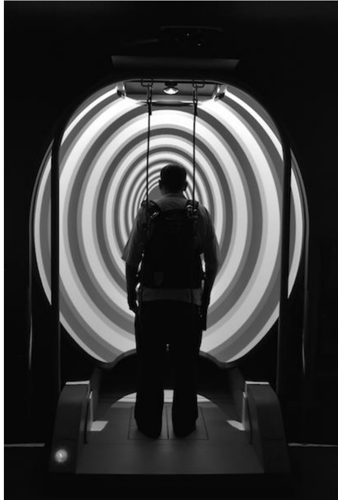
Fig 3. Participants were fitted with a safety harness, placed on a stable platform, and exposed to computerized dynamic posturography with immersion virtual reality.
