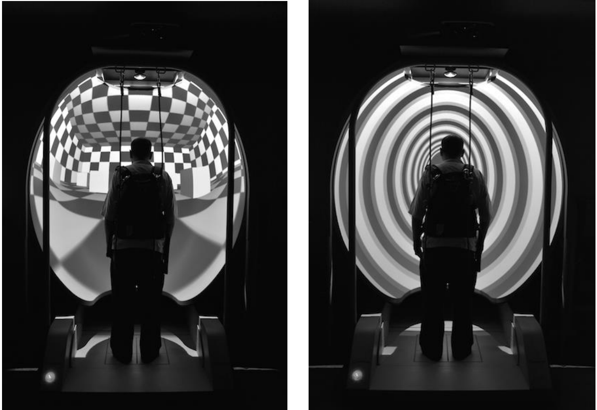
Fig 1. Participant was fitted with a safety harness, placed on a platform, and exposed to Computerized Dynamic Posturography with Immersion Virtual Reality. Condition 1: stable platform, eyes open, and stable visual scene (left); Condition 2: stable platform, eyes open, and infinite tunnel visual flow (right).
