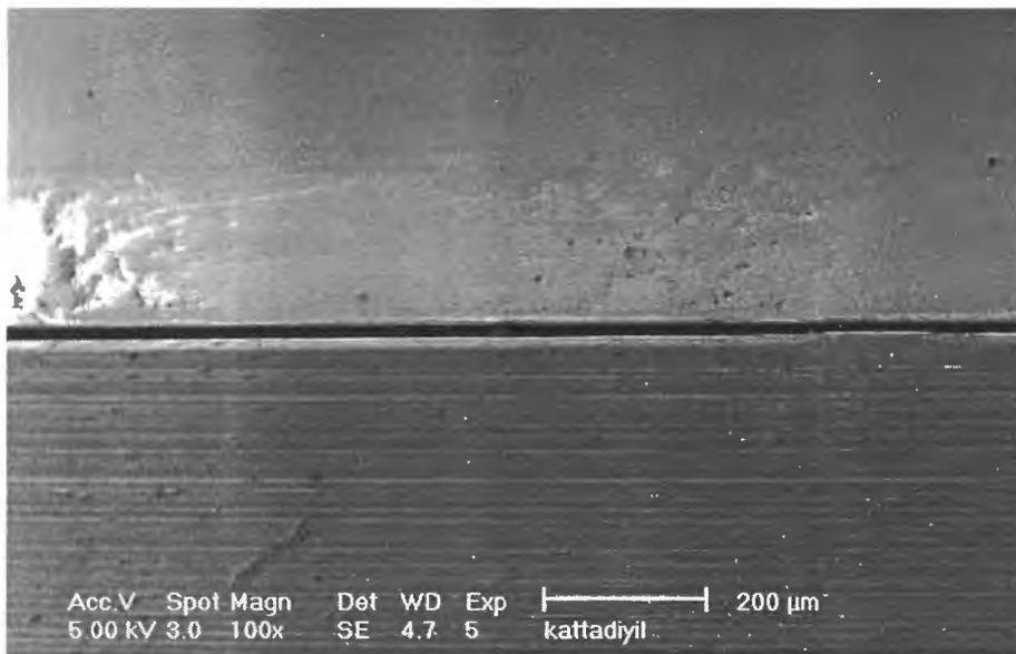
**Figure 6: Scanning Electron Microscopic view of the Finished Cast Plastic Implant Innovations Abutment-Implant body Interface**
