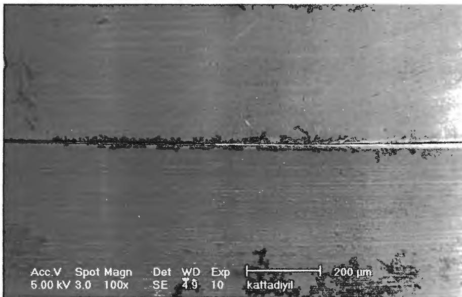
**Figure 4: Scanning Electron Microscopic view of the Cast Gold Implant Innovations Abutment-Implant body Interface**
