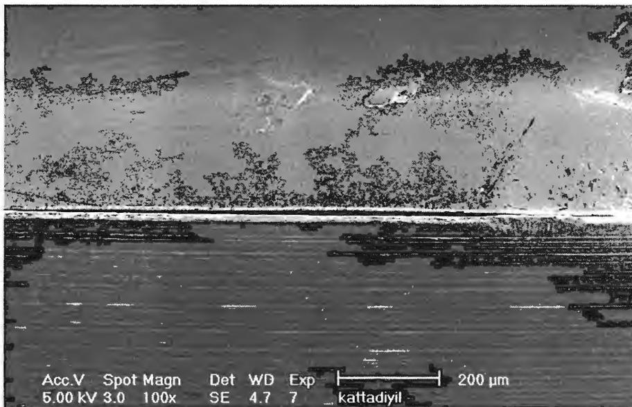
**Figure 3: Scanning Electron Microscopic view of the Cast Gold Nobel Biocare Abutment-Implant body Interface**
