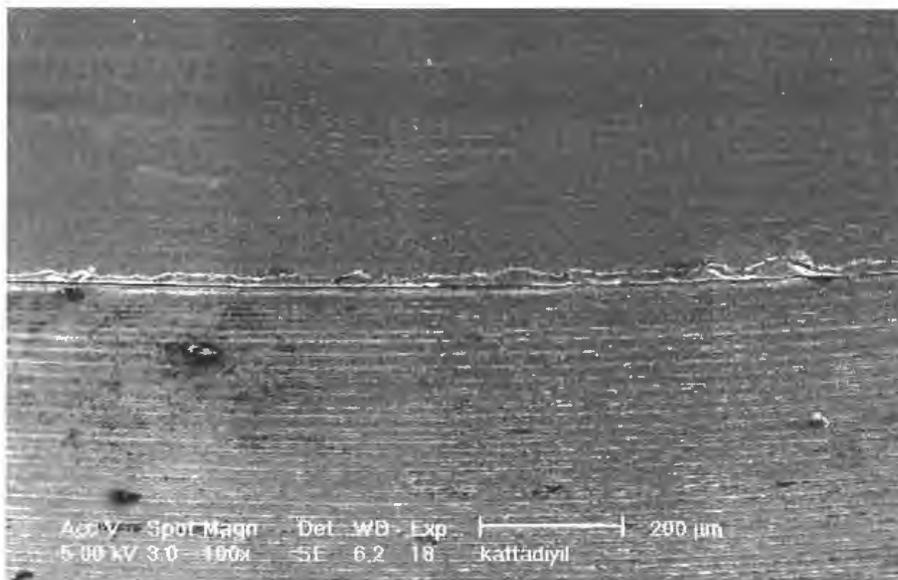
**Figure 8: Scanning Electron Microscopic view of the Procera™ Nobel Biocare CAD-CAM Abutment-Implant body Interface**
