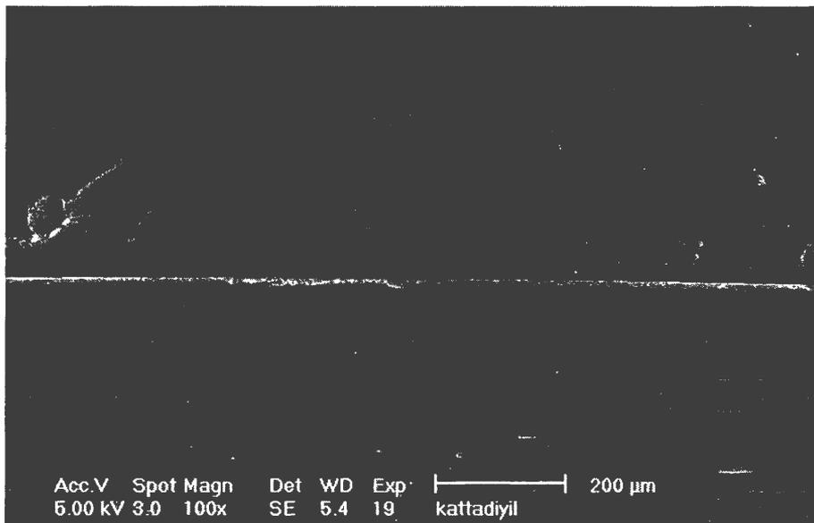
Figure 5: Scanning Electron Microscopic view of the Finished Cast Plastic Attachments International Abutment-Implant body Interface
