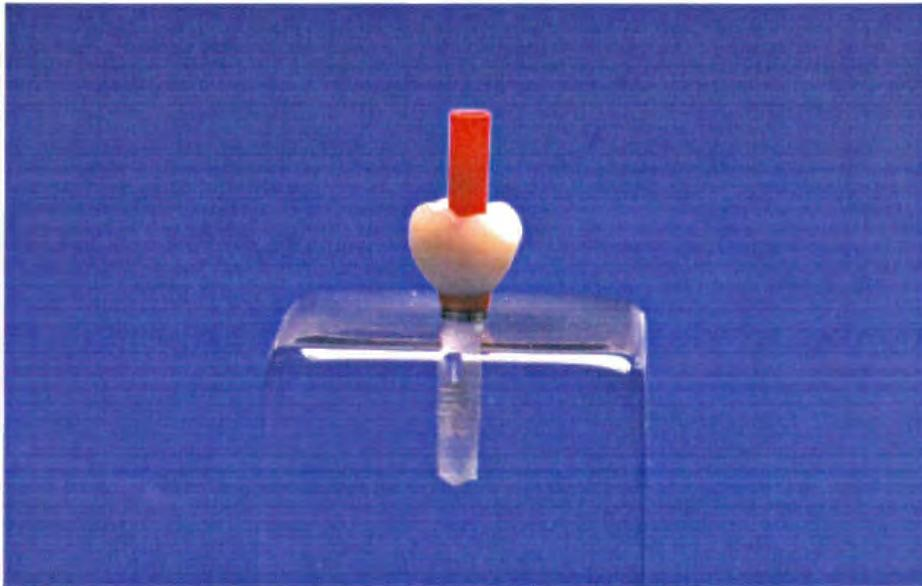
Figure 2: Standard wax pattern used for duplication
