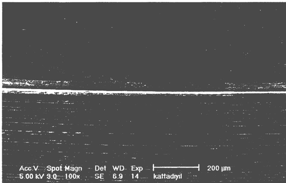
Figure 7: Scanning Electron Microscopic view of the CeraOne® Nobel Biocare Abutment-Implant body Interface
