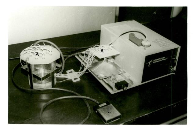
A = Pressure reservoir jar; contains tubes of the phage dilutions
