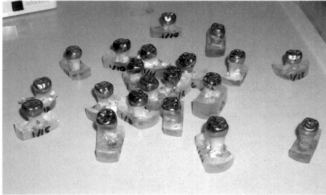
Figure 2.1. Twenty completed stainless steel crowns.
