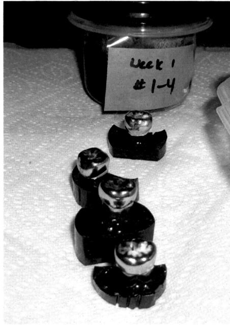
Figure 2.2. Specimens, with nail varnish, prior to dye immersion.
