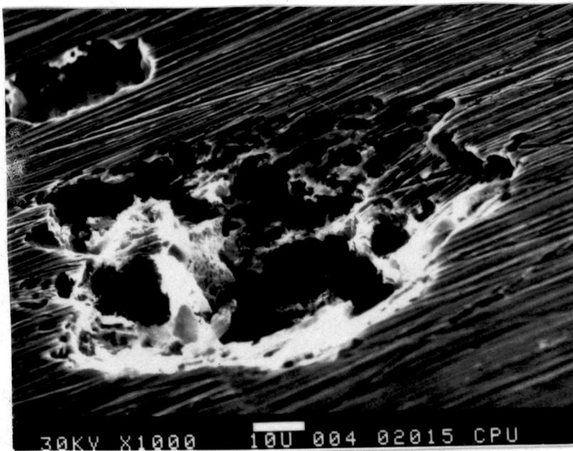
(figure 5--Scanning electron micrograph showing an open pore on surface of powdered metal sample. Original magnification, X1000)
