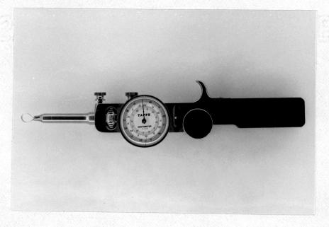
Figure 1. Dentometer used for measuring the circumference.
