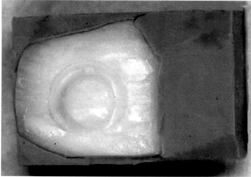
Figure 1 - Mounted tooth in block, pre-staining. Note 4-mm diameter test area.
