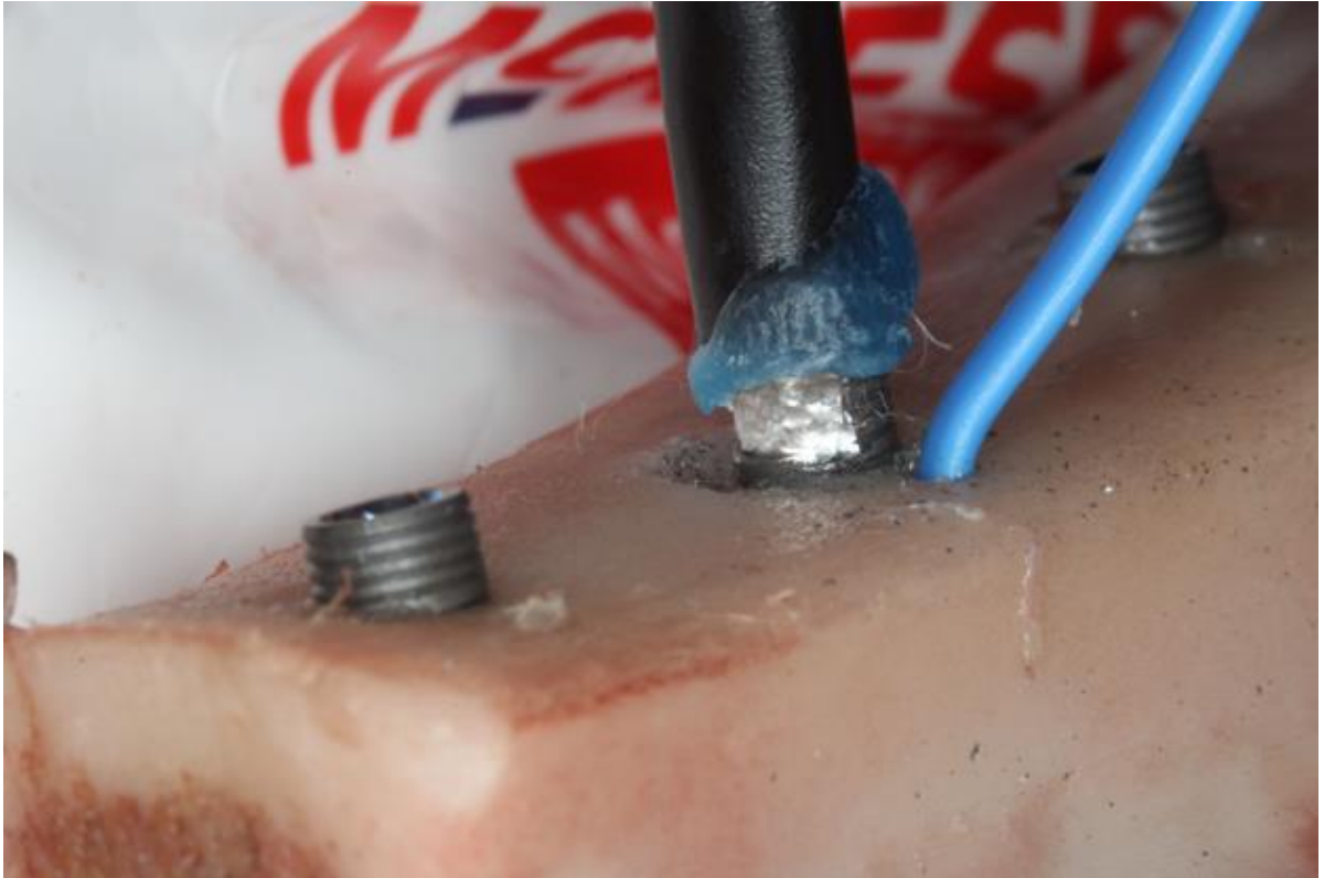
Fig 4. Wax used to seal openings around thermocouples to isolate thermocouples from irrigation during implantoplasty.
