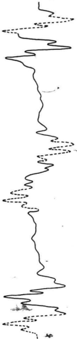
FIGURE III - 8 ESR SPECTRUM SHOWING CENTRAL CONTRIBUTION OF WING STRUCTURES
