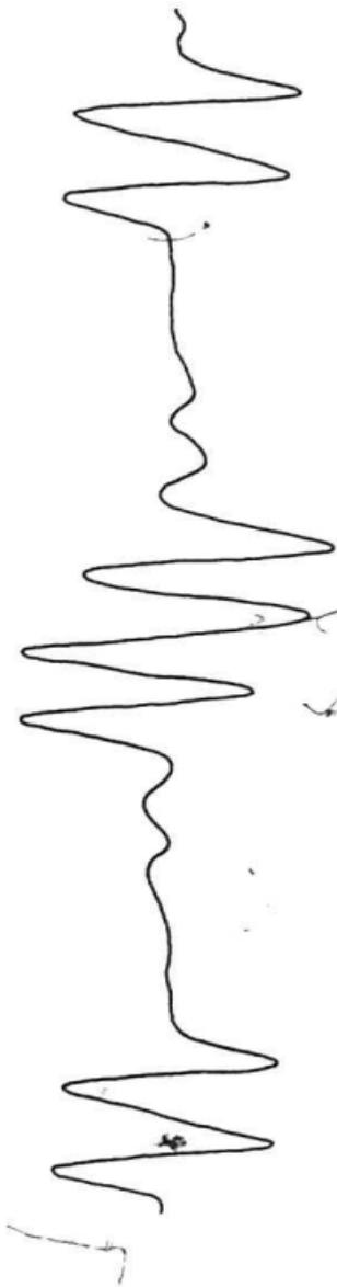
FIGURE III - 6 ESR SPECTRUM WITH SIMPLE ABSORPTION LINE SHAPE
