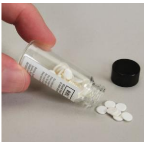
Figure 3. 6mm diameter sterile discs (antibiotic sensitivity disks, blank, sterile, Carolina Biological Supply Company, Burlington, NC, USA)
