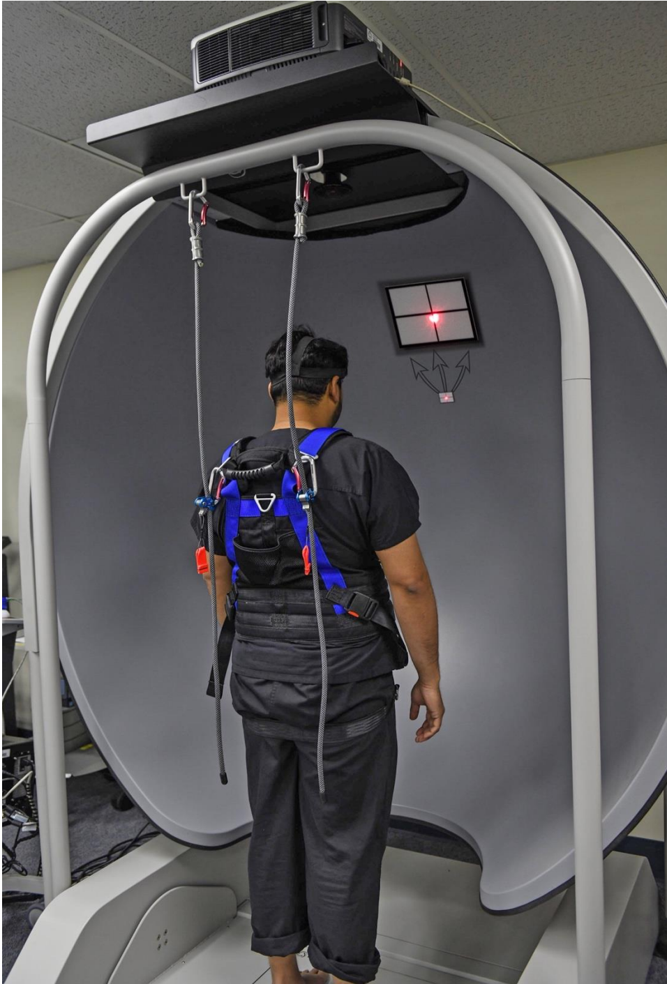
Fig. 3. CDP-IVR dynamic conditions 1-5 Participants performed horizontal and vertical head motions using the showing head-mounted laser pointer and amplitude grid (grid magnified for easier reader viewing).
