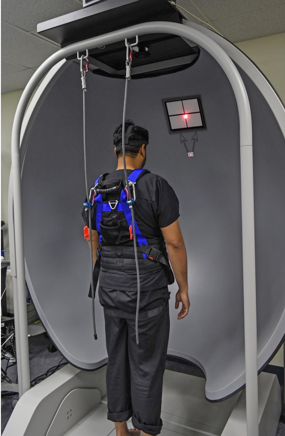
Fig. 3. CDP-IVR, laser pointer over subject head, the grid pic.is magnified to be easy to see, This demonstration for head motion conditions 2, and 3.
