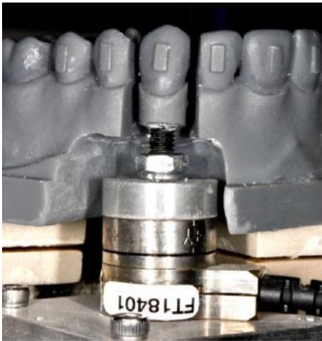
Figure 3. Canine tooth fastened to ATI Industrial Automation load cell (Nano-17-E).
