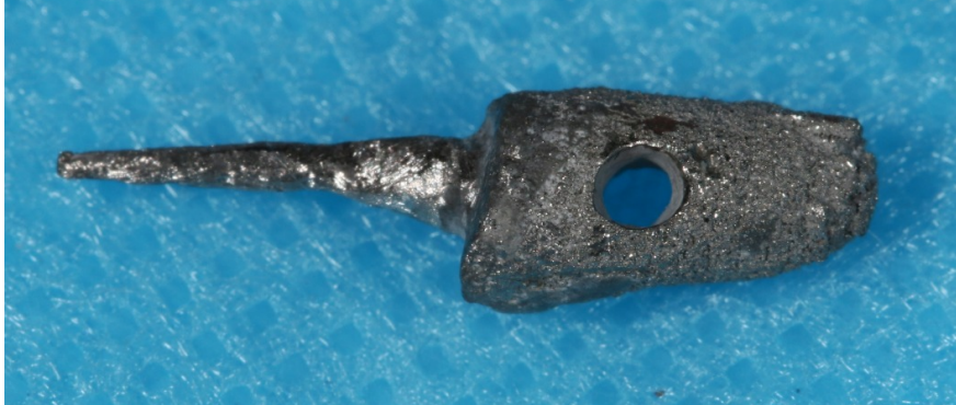
Figure 8. Custom printed post-and-core (Titanium) alloy with hole
