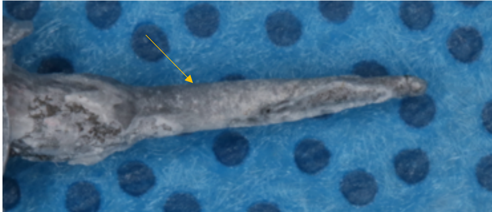
Figure 17. Cohesive failure at post/root interface in relined sample (Arrow)
