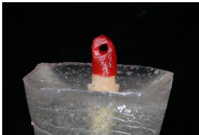
Figure 4. Acrylic resin post build up and the hole made to prepare the post for pull out test
